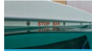
Rear Stop Bar stops the paddlewheel in an emergency.
